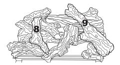
Figure 47 - Installing Logs No. 8 and No. 9
